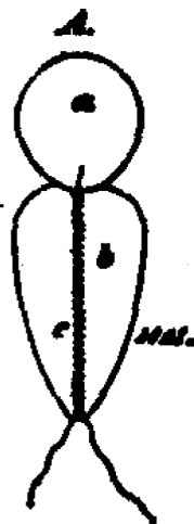
Fig. 2-1. Phone used for transmitting and receiving; "a" is metal contact; "b" is handle; and "c" is wires going through the handle. (New York Public Library)
